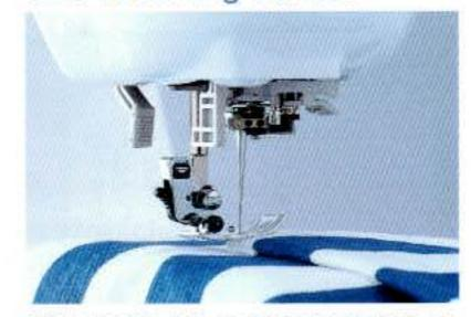
This keeps the presser foot level so that smooth seams can be obtained when sewing at the beginning of stitching.
