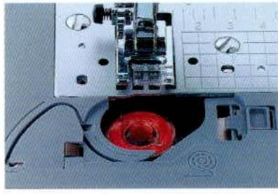
Simplicity itself. Insert the bobbin and pass the thread in the direction of the arrow. Start sewing.
