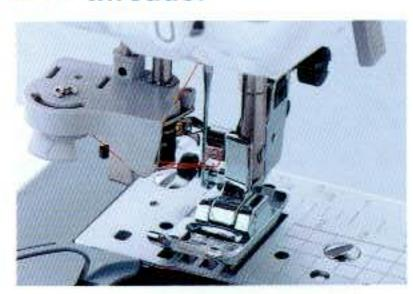
Quick and easy needle threading.
