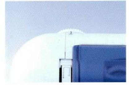
When sewing stretch fabrics, the degree of pressure exerted by the presser-foot prevents the material being stretched.
