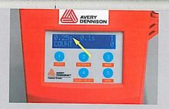
Increase machine output with actuation speed programmability. Choose the best speed for your application – as fast as .25 seconds/staple vs. .45 seconds/staple for other systems to maximize productivity. Or, choose a slower cycle, .60 seconds/staple to penetrate maximum layers of denim.
