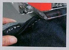
Make whiskering faster and easier than ever, thanks to superior fastener strength and a double-shot feature that installs two fasteners in one cycle.
