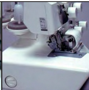
Differential Feed Dial is controlled and adjusted by a dial conveniently located on the outside, left-hand side of the machine (MO-644D-only)
